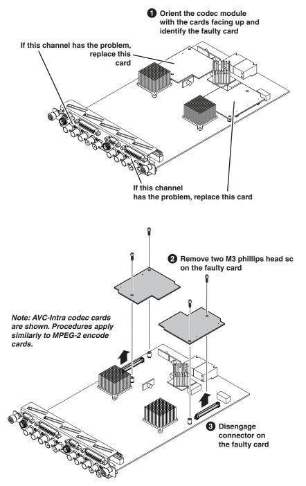
After installing the replacement card, install the current version of K2 software. An over-install is all that is required. You do not need to first un-install the software. This ensures that the card is flashed with the proper version to be compatible with K2 software.
