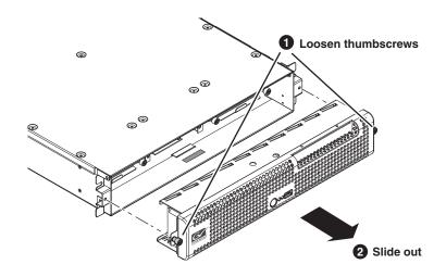
You can remove the bezel assembly while the K2 Summit Client is operating. If you do so, make sure you replace it within three minutes to ensure that the correct operating temperature is maintained.
