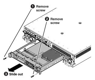
When replacing the carrier board, the screw attachment sequence is critical, as illustrated.
