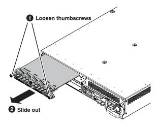
A CAUTION: Improper removal can damage components on the board. Make sure you slide the board straight out. Do not allow the back end of the board to bang up against the lid after it is no longer secured by the card guides.
