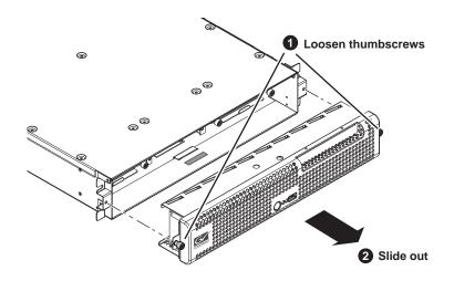
You can remove the bezel assembly while the K2 Summit Client is operating. If you do so, make sure you replace it within three minutes to ensure that the correct operating temperature is maintained.
