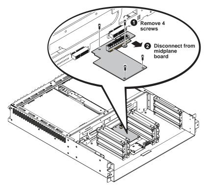
When installing the disk controller board, orient as illustrated.
