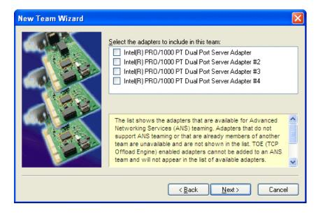
7. Select the check box for the adapter name that maps to Control Connection #1 (PCI bus 4, device 0, function 1) and for the adapter name that maps to Control Connection #2 (PCI bus 3, device 0, function 1). Click **Next**.
