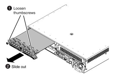
NOTE: With a firm grip on the metal (EMI) bracket, ensure the board is level and parallel to the card guides to avoid damage to the components on the edge opposite the rear panel.
