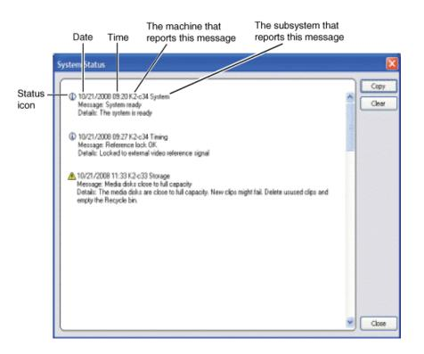
The StatusPane is used to view detailed system messages including status, warning, and error messages. System status messages provide status icons and a description of the status event reported by the message. If there is a problem, a corrective action is indicated. Use these messages along with troubleshooting problems to determine if a service procedure is necessary.
