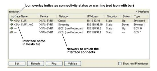
The devices under that node are displayed in the device list view and the interfaces on the devices are displayed in the interface list view.
