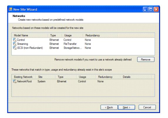
The Networks page displays a list of networks that are defined for the selected site model. Each of these networks is based on a network model that defines the type, usage and redundancy of the network. When the New Site Wizard creates a network, it is based on this model.
