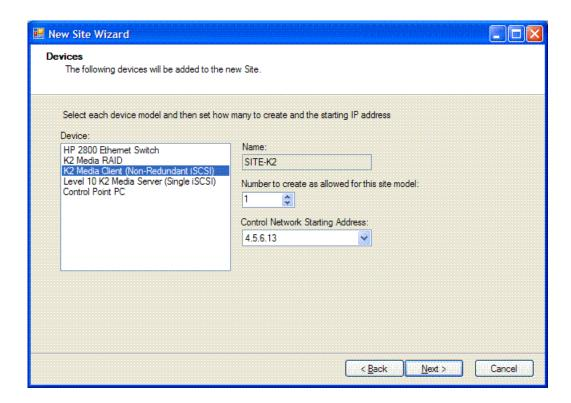
The Devices page shows you the device models that typically comprise a site based on the model you chose in the first page of the New Site Wizard. The New Site Wizard creates these devices as part of the site. You can then modify, remove, or you add devices, including device models that are not shown on this page.
