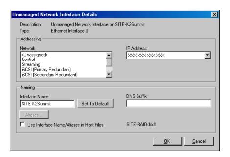
The Unmanaged Network Interfaces dialog box allows you only to save changes to the system description.
