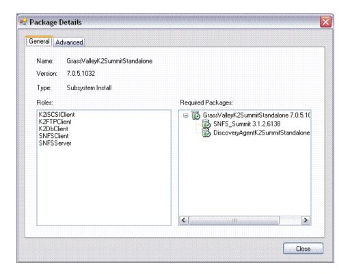
From this dialog, you can view which software installs are contained within the managed package and whether or not there are any software dependencies. You can also see the software roles that this package contains. Deployment tasks are generated if the following two conditions are fulfilled:
