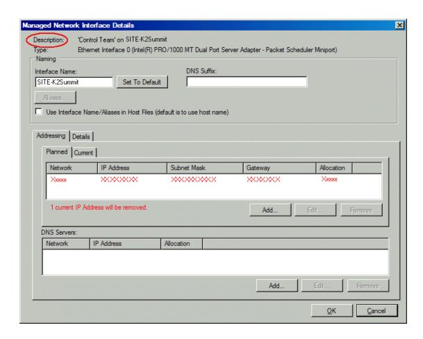
The Managed Network Interfaces dialog box allows you to edit and save changes to the device.
