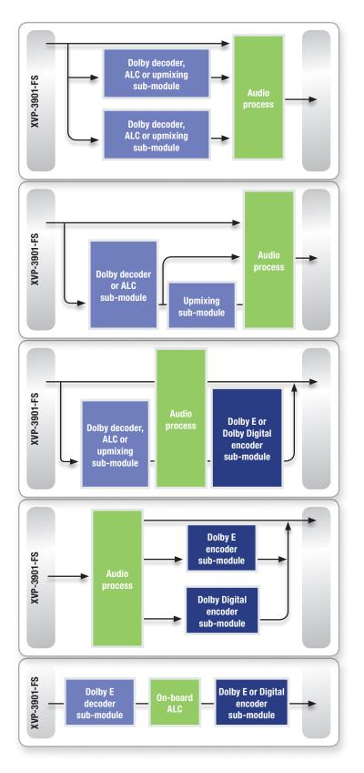
Dolby E / Dolby Digital (AC-3) decoding, automatic loudness control (ALC) or upmixing (or a different combination of these sub-modules) used in parallel ahead of audio processing.
