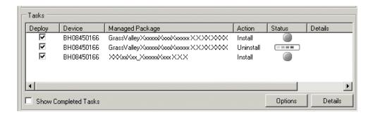
Deployment tasks run and software is uninstalled. Progress is reported and next steps are indicated in both the Status and Details columns. If an error appears regarding prerequisite software, install the prerequisite files on the control point PC and then repeat this step.
