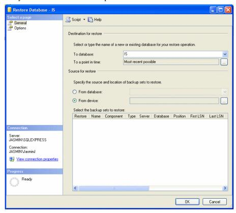
6. In the Destination for restore section, select IS from the database dropdown list. Key in "IS" if it's not in the dropdown list.
