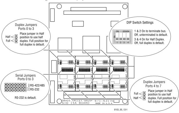
Figure 1. SIO ISA Port Jumpers and DIP Switches
