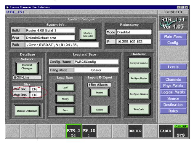
This illustration assumes we want to configure 128 destinations, 128 sources, and eight destination monitors. In this case the number of destinations is increased by eight from 128 to 136 to incorporate the eight destination monitors. The number of sources is also increased by eight to maintain a symmetrical configuration.
