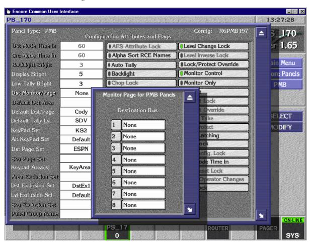
7. Since XY and 48B panels can control a single destination at a time a single destination can be monitored, the attribute DstMonitor/Page can be assigned to the configured destination Monitor. See Figure 18.
