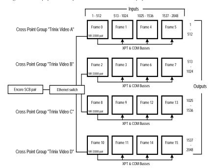
Figure 6. Simplified view of Encore Cross Point Groups for Trinix 2048 x 2048 router.
