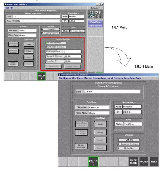
The DB Name cannot be changed if the Panel Server is in the Mirror mode. It uses the same DB Name as that of its Master.
