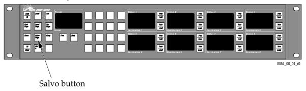
With Encore 1.6.5.1, a Salvo mode button has been added to the PMB assignable button functions. This button functions the same as the Salvo mode button on the XY panel; i.e., when the Salvo mode button is pressed, the level display shows ^SALVO^.
