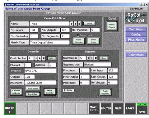
*Figure 7. Example of Trinix configuration settings for 128 x 128 router.*
