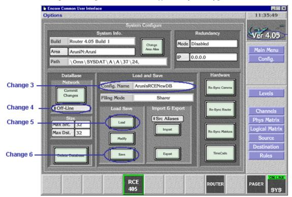
Figure 28. Changes to Router Controller application System Configuration screen
