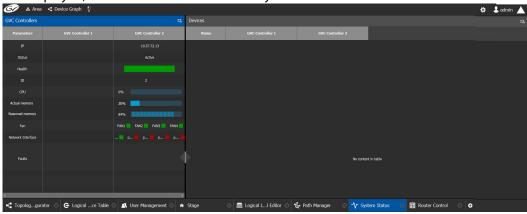
• [Ref. #PEG-9078] **Densite Conrol Ports are now active on the inactive GV Convergent server:** on the system status page inside the GV Convergent Client, the Densite Gateway control points would status as 'Standby' on the inactive controller. They were standby until the release of GV Convergent 1.7.0. Those control points are now active on the inactive controller and will status accordingly. This improvement will allow for shorter fail over times between GV Convergent controllers.
