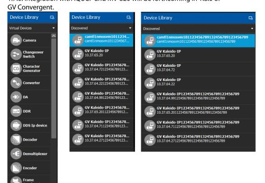
• [Ref. #PEG-9133] Initial SAM integration added to GV Convergent: SAM IQMIX can now be discovered and added to the topology within GV Convergent. For the 1.7.0 release, only SAM devices can be routed to other SAM devices to accommodate other integration efforts that are forthcoming in future releases.
