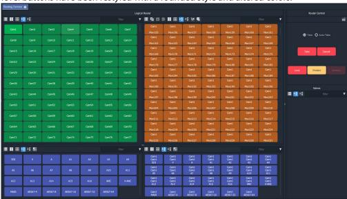
• [Ref. #UCCM-1118] **Lock and Protect destinations support in the Bulk Routing:** Added support to Lock and Protect destinations. *Lock* and *Protect* applies to all levels associated with the destination. Protected destinations and their levels are indicated in yellow. Locked destination and their levels are indicated in red.
