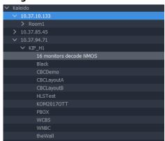
Expanding a Kaleido multiviewer in the GV Orbit client network tree will cause GV Orbit to connect to the device and obtain a room listing which will be displayed as child nodes in the tree. Under the rooms layouts will be displayed.
