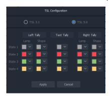
• [Ref. #UCCM-1894] **Ability to Easily Assign TSL Value to Widget:** Added feature to enable the user to quickly assign TSL functionality to Tally Lamp, Label and Shape Widgets. Select the widget, right click and select **TSL configuration**. Select the source of the tally, e.g. left or right tally. Select the TSL address level, e.g. L1, L2 etc. If the user has renamed the levels then their custom labels will be shown.
