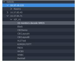
Expanding a Kaleido multiviewer in the GV Orbit client network tree will cause GV Orbit to connect to the device and obtain a room listing which will be displayed as child nodes in the tree. Under the rooms layouts will be displayed.
