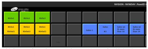
Added Support for 24 Character Display on NVision Panels: Added 24 character support to the Category, Load page and Load layout buttons. This is regardless of the Display 24 characters property as these buttons only display the name of the element.
