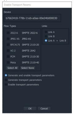
To automatically set multicast parameters select Enable Flows, configure the flow types and select the desired mode.
