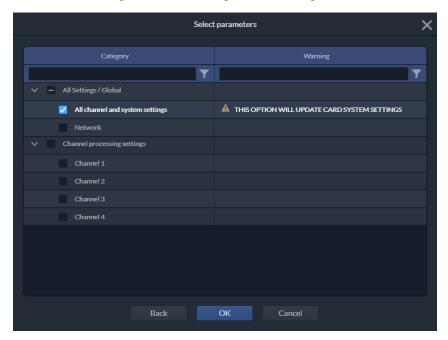
Selecting the All Channel and System Settings option will recall all operational settings for the card and all of its processing channels.
