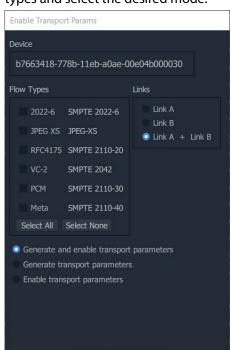
To automatically set multicast parameters select Enable Flows, configure the flow types and select the desired mode.
