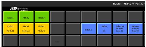
Added Support for 24 Character Display on NVision Panels: Added 24 character support to the Category, Load page and Load layout buttons. This is regardless of the Display 24 characters property as these buttons only display the name of the element.
