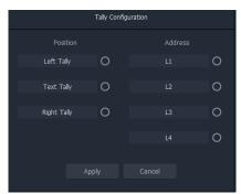
• [Ref. #UCCM-1893] **Global Configuration of TSL Addresses:** Feature added to Multiviewer Room Editor to enable user to configure TSL addresses associated with each Multiviewer destination. The user can assign up to four TSL addresses per destination. The default address level names, L1, L2, L3 and L4 can be modified by the user.
