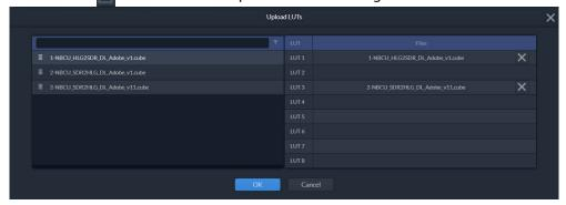
The list of available LUT files can be filtered. Use the drag handle to drag and drop the file into the appropriate slot. Up to eight slots can be populated. After clicking OK the LUT files will be uploaded to the respective slots on the selected devices.
