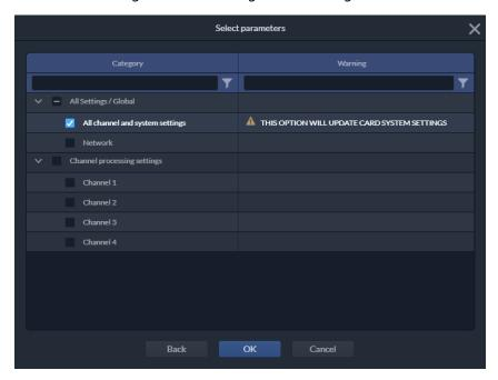
Selecting the All Channel and System Settings option will recall all operational settings for the card and all of its processing channels.
