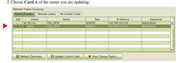
If you are updating an expanded NV8576-Plus, you must select **Card A** of the master frame. MRC will present a dialog asking you to identify the slave frame. Choose the slave frame in this dialog. (But do *not* select the slave frame in the 'Control Cards' tab at the bottom of the 'Module Types' page!)
