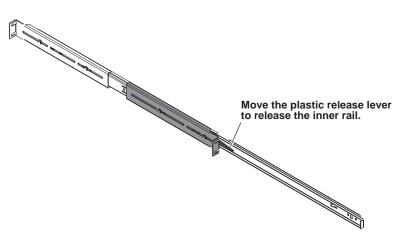
The plastic release lever moves up on the left-hand rail and down on the right-hand rail. You might need a slotted screwdriver to move the plastic release lever.
