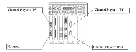
HD/SD model with no recorder channels, two player channels:
