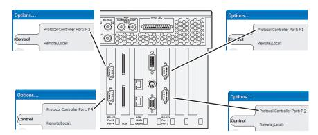
Remember that in the context of the Protocol Controller Port reported in the Options dialog, the labels P1, P2, P3, and P4 refer to RS-422 rear panel connectors (ports) 1, 2, 3, and 4, *not* Player Channels 1, 2, 3, and 4
