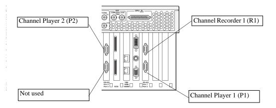
HD/SD model with no recorder channels, four player channels:
