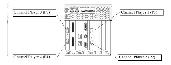
HD/SD model with no recorder channels, three player channels:
