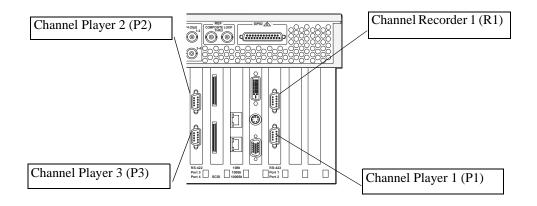
HD/SD model with one recorder channel, two player channels:
