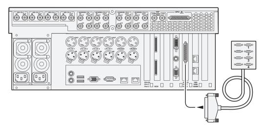
• **Direct-connect storage** — There is a new model of K2 Media Client, with its own external RAID storage directly connected. Like a K2 Media Client with internal storage, this model is referred to as "stand-alone" storage, as opposed to K2 Media Clients that connect to external shared storage.
