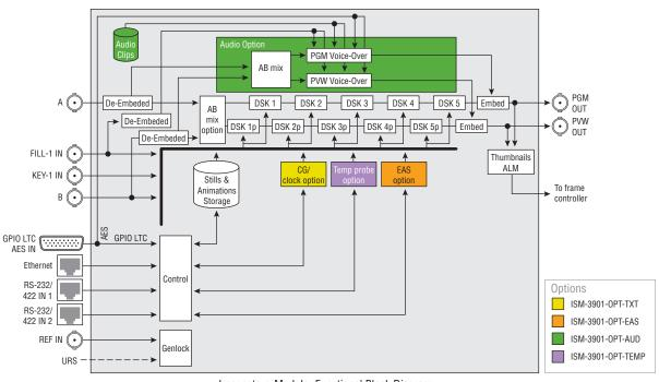
Imagestore-Modular Functional Block Diagram
